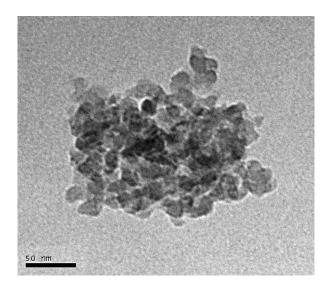
*S-Figure 3.* TEM image of the calcined silylated nano faujasite sample
