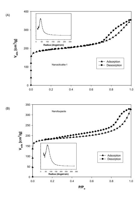
*S-Figure 2.* Nitrogen adsorption/desorption isotherms and BJH pore radius distribution (inset) of the calcined nanosilicalite-1 and nanofaujasite samples
