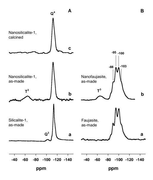
*S-Figure 1*. <sup>29</sup>Si MAS NMR spectra of the as-made silvlated samples prepared from the same zeolite gel, in solvent medium in the presence of organosilane, and in aqueous medium in absence of organosilane, respectively.
