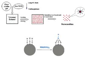
surface. An organic solvent is used as the medium for crystallization instead of water. The zeolite precursors are functionalized with organic silane groups. They thus become hydrophobic and highly dispersed in the organic solvent. Because the crystallization occurs in the organic phase and the zeolite precursors are protected by functional groups, catastrophic aggregation can be prevented hence, resulting in small and uniform nanozeolites with hydrophobic external surface.
